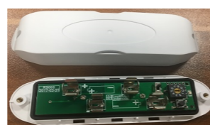
Lift outer cover from circuit board
