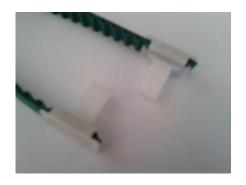
• Attached the white "belt to carrier" anchors to each END of the belt.
