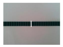
• Attach the white "belt to carrier" anchors, one each side of the belt centre line.
