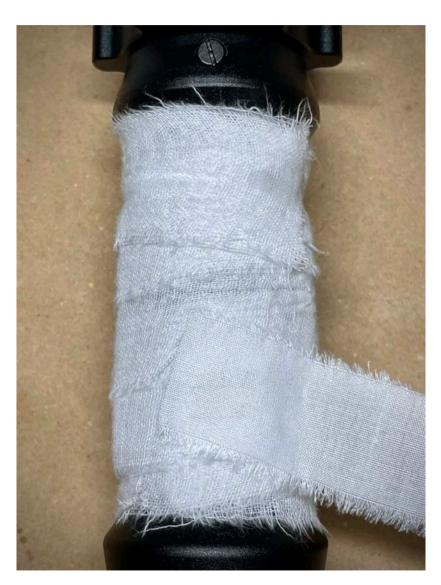
For the second part of the wrap, provided in the wrap kit are three different white fabrics, this one is the same length as the previous strip we used, but is thicker.
