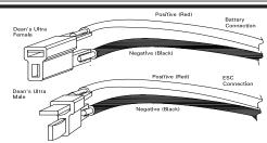
Caution: Battery and ESC connections must follow standard convention as above. All batteries must be at full charge before connection.
