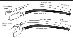
Caution: Battery and ESC connections must follow standard convention as above. All batteries must be at full charge before connection.
