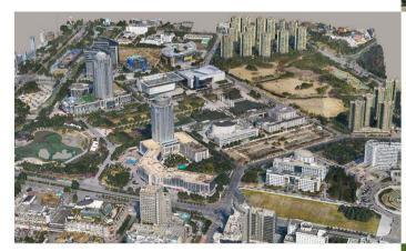
To create a smart city, high-resolution remote sensing images from multiple angles of the city or key areas can be obtained by using UAV tilt photogrammetry, and the real 3D model of the city can be automatically generated.
