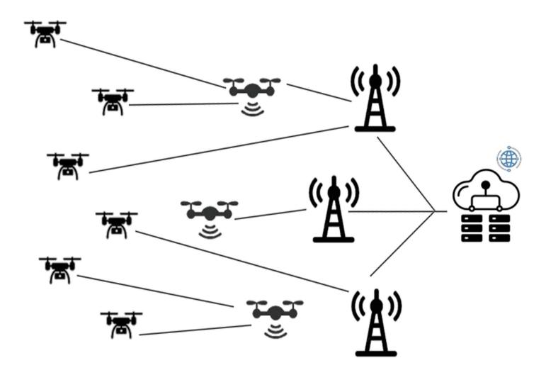
A single node supports communication with up to 64 devices. Users no longer depend on network operators, and can completely set up ground base stations and relay stations independently. The running devices can realize roaming communication between different base stations, so as to achieve full coverage of the area, which is especially applicable for scenarios that require batch deployment and cluster control.
