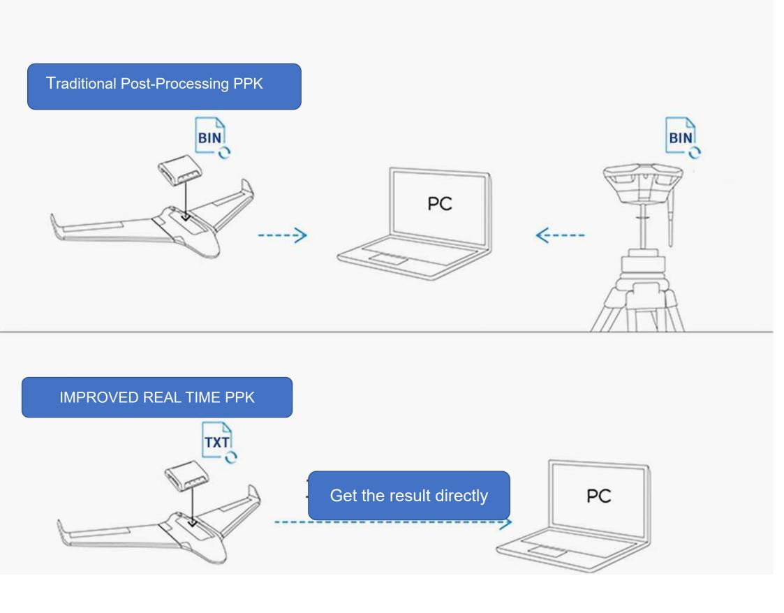
In the field of aerial surveying and mapping, the traditional PPK post-processing technology is to record the data of the mobile terminal and the base station for calculation. This process depends on the quality and integrity of the satellite data. If there are problems that cannot be found in time, it may bring losses to users.
