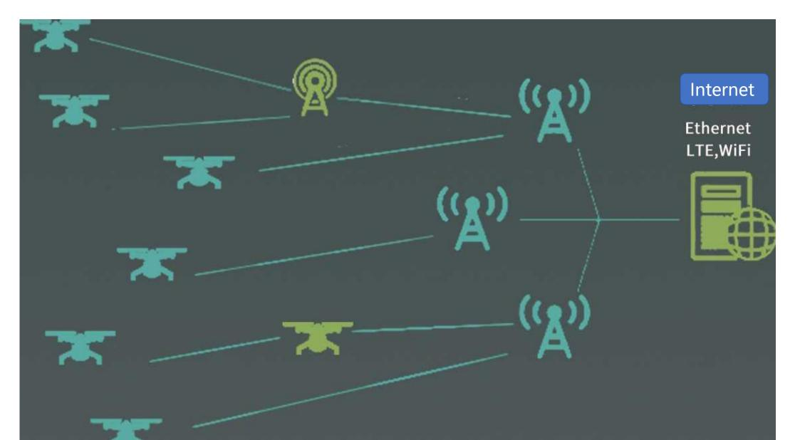
A single node supports communication with up to 64 devices. Users no longer depend on network operators, and can completely set up ground base stations and relay stations independently. The running devices can realize roaming communication between different base stations, so as to achieve full coverage of the area, which is especially applicable for scenarios that require batch deployment and cluster control.
