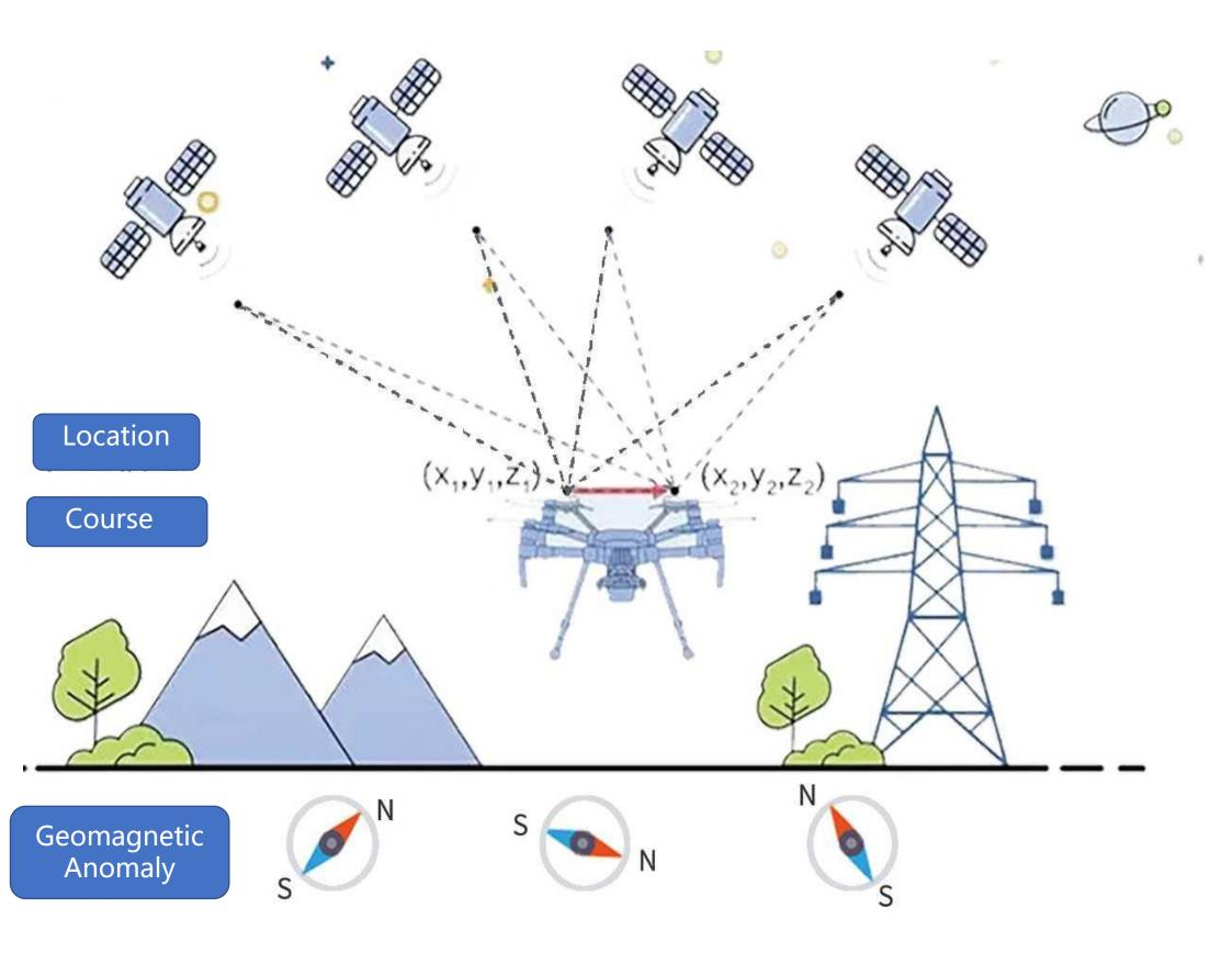
The dual-antenna direction-finding technology means that the master-slave two antennas form a baseline vector, and the angle between the baseline direction and the true north direction is obtained through differential analysis, so as to obtain the current heading of the aircraft, which can replace the magnetic compass for UAV navigation. Meet the application requirements in special environments such as power inspection and pipeline inspection.
