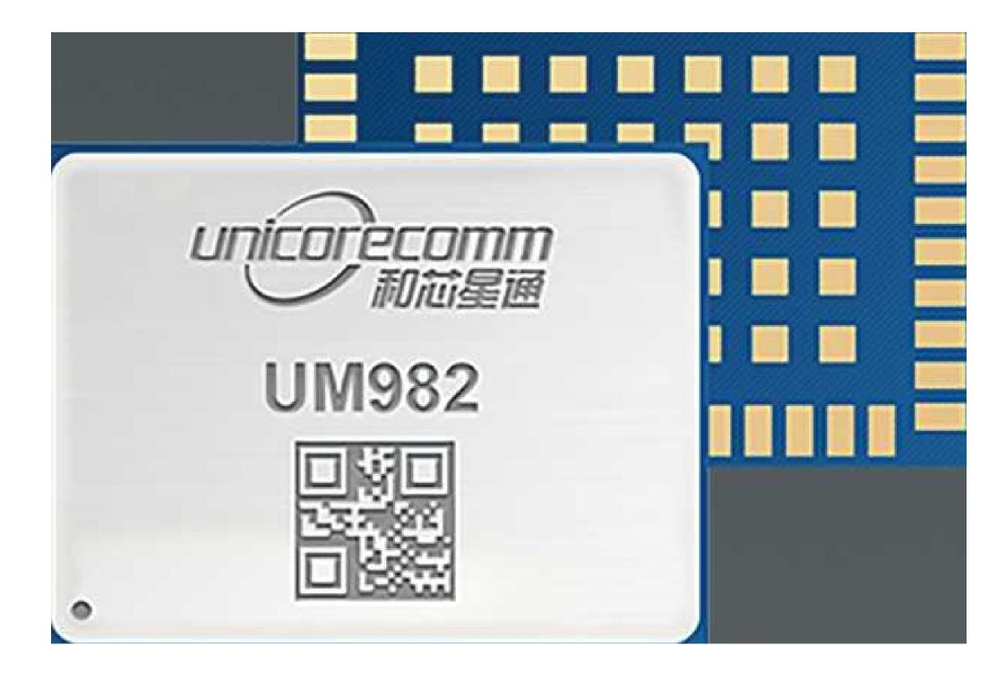
It adopts the new generation of BDS/GPS/GLONASS/Galileo/QZSS high-precision positioning and orientation module independently developed by Unicore, based on the new generation of radio frequency baseband and highprecision algorithm integrated GNSS SoC chip-NebulasIV design. The built-in advanced antiinterference unit ensures that the module can provide reliable and accurate positioning accuracy even in complex electromagnetic environments.
