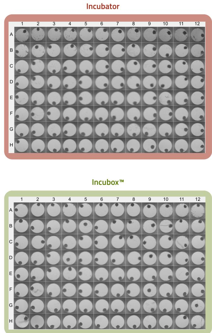
**Figure 5:** Plate scans showing brightfield images of individual wells at day 5. Increased evaporation in standard incubators (upper scan) causes morphological changes of microtissue and precipitations in outer wells (row A). No morphological changes are visible in plates cultured in the Incubox™ (lower scan).
