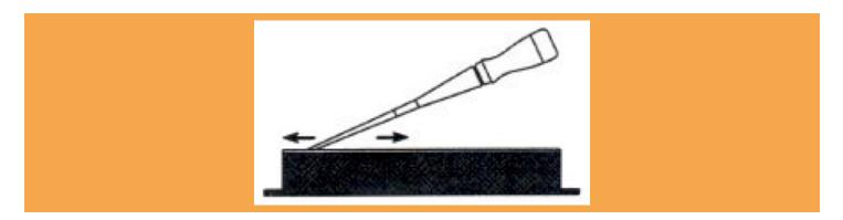
When you've done that, flip the chisel over again, and pull backwards to remove the fine burr. You might find that another smaller burr is then created on the bevel side. Alternate between back and bevel until the burr is completely gone.
