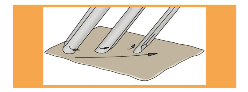
Use your strop to remove any final burrs and polish your finished blade. Remember to strop both the inside and outside of the gouge.
