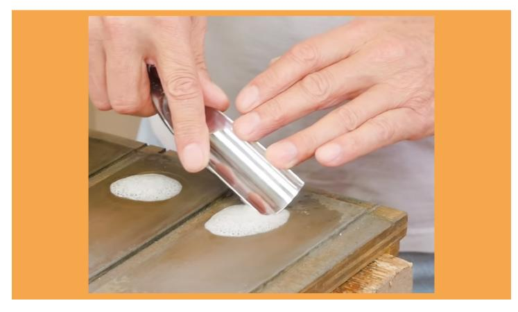
Continue this until you see a small metal burr (the small fold of metal that forms at the apex of the cutting-edge during sharpening) on the inside edge of your gouge.
