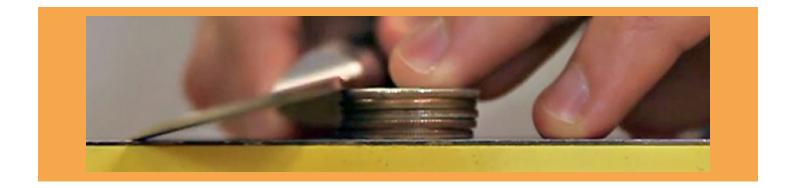
Pull the bevel back along the 400# grit side of the stone, putting pressure on it with your fingers. Continue that until you have a nice straight pattern of scratched running along the bevel. You should be able to feel a burr across the whole width of the edge.
