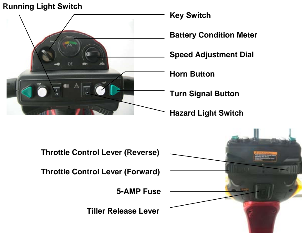
FIGURE 6 & 6A. TILLER CONSOLE
