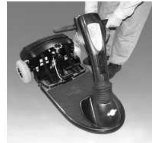
FIGURE 10A. LOWER THE TILLER
