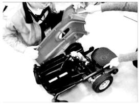
the front end of shroud for matching with the front frame. (one for each LH and RH) (Fig D4)
