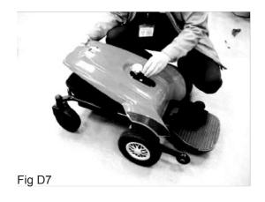
4. Slightly lean down the front end of shroud. This will make the seat post go through the hole at the shroud center. (Fig D7)
