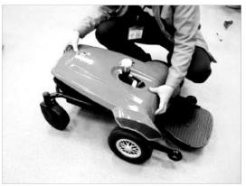
5. Make sure the shroud front end touches the front frame and then slightly move the shroud from rear to front. This will make the front hooks attach to the bracket at the frame. (Fig D8)
