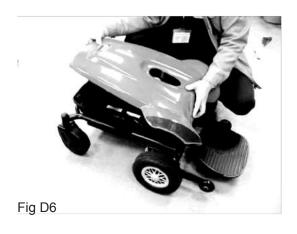
3. Use two hands to hold the front end and rear end of the shroud. Align the hole at the shroud center with the seat post. (Fig D6)
