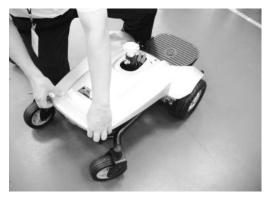
1. Use two hands to hold the rear end of the shroud. Slightly pull up the rear end of the shroud. This will release the rear hooks from the bracket at the battery tray.(Fig D1)
