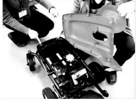
2. Please note there are two hooks at the rear end of shroud for matching with the battery tray. (one for each LH and RH). (Fig D5)
