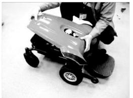
2. Holding it the same pull the shroud up, this will release the the front hooks from the bracket at the front frame. (Fig D2)
