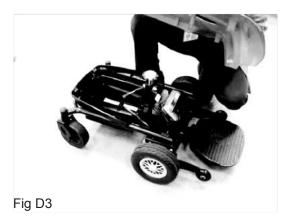
3. After both hooks are released from the front frame and rear battery tray, it can be removed from the base unit. (Fig D3)
