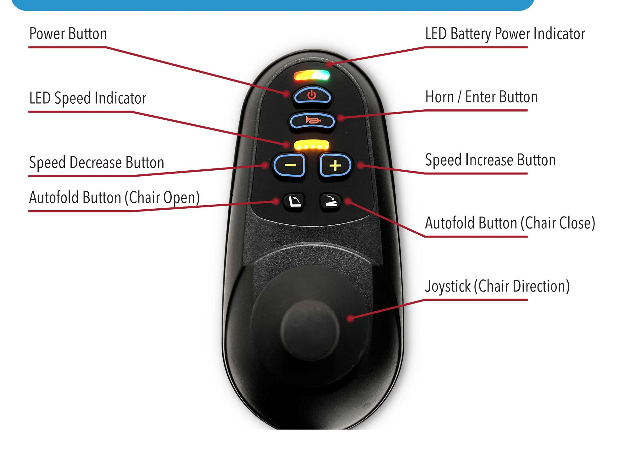
**Power Button:** To turn on the chair, press the power button. To turn it off, press the button again. When the chair is powered on, the LED Battery Power Indicator will light up.
