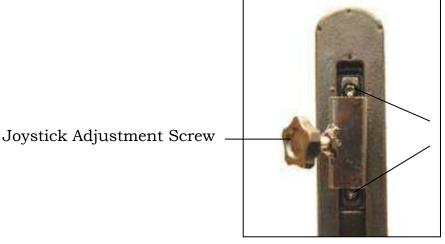
Joystick Bracket Bolts (2) (5mm Allen)
