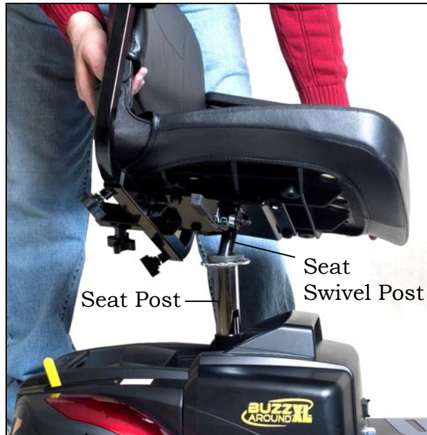
Figure 23. Installing the Seat
