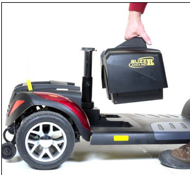
Figure 21. Battery Pack Installation
