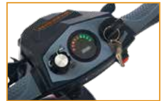
LED battery indicator on the console
