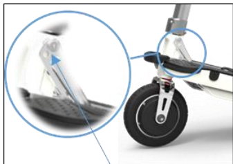
Figure 22 Steering Rod angle adjustment screws
