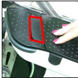
Figure 56 - battery release button
