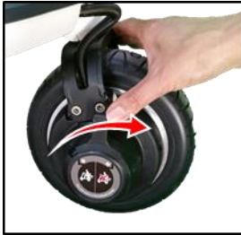
Figure 51 Releasing the freewheel
