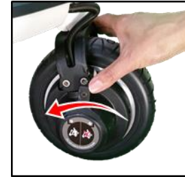
Figure 52 Securing the freewheel
