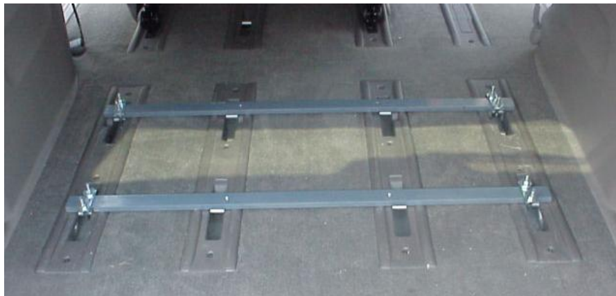
Example: Mounting Bars Installed
