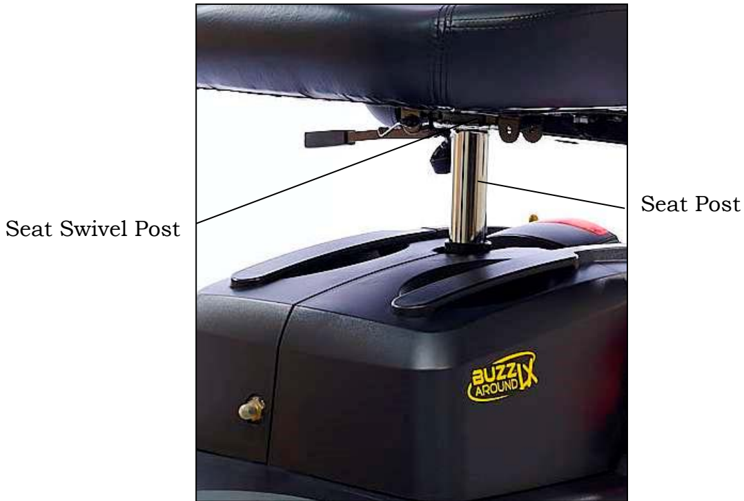
Figure 25. Installing the Seat
