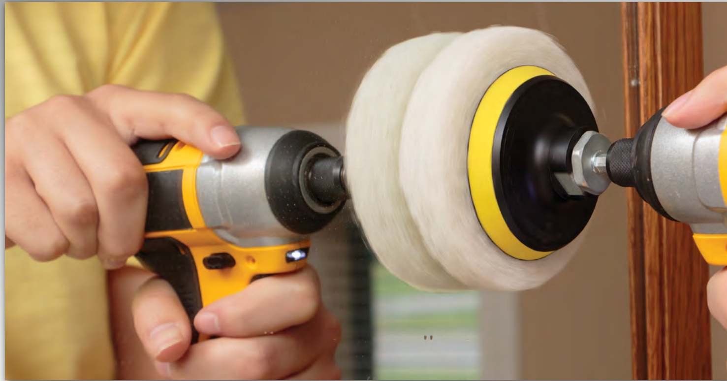
Threaded-to-Quickchange Adapter in a 3 inch Backer attached to a White 4 inch pad scrubbing a mirror.
