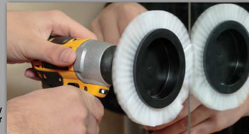
Soft White Edge brush getting in the crease between two panes of a bathroom mirror.
