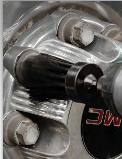
Ultra Stiff 1 inch Long brush being used on lug nuts.
