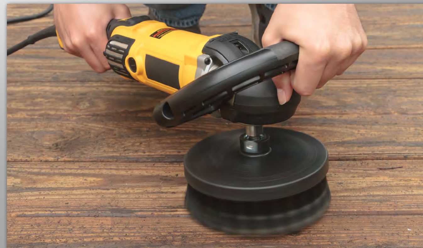
Ultra Stiff 7 inch brush scrubbing deck planks
