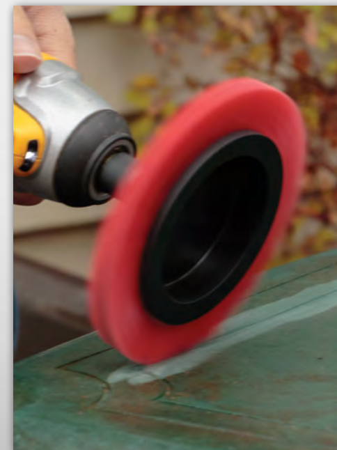
Stiff Edge brush cleaning trimwork on a plastic patio table.
