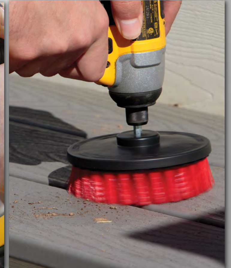
Stiff Red 4 inch Drillbrush scrubbing deck stairs.
