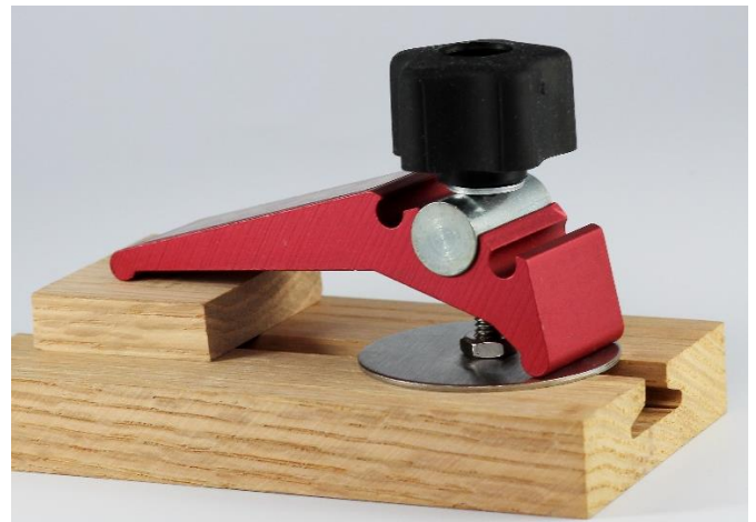
A knee-style hold-down clamp with a 2-1/2” threaded post
