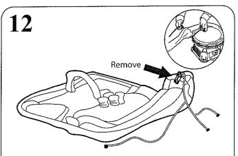
Untie the drawstring from the short Outlet Tube and allow the Water Park to fully deflate. Remove the Hose Assembly from the arch and wrap it up with no kinks.
