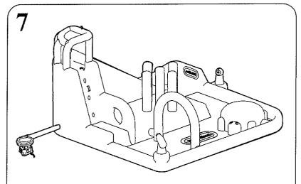
Water Park will inflate in 2 - 3 minutes. Blower should remain on to continuously inflate the Water Park during use. Air flow through seams is normal. Do not try to repair or seal seams NOTE: You may need to lift the yellow arch to help it stand up.
