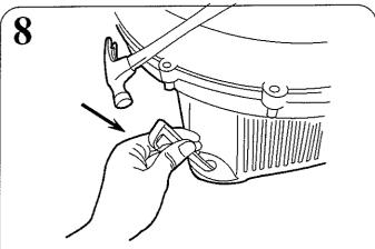
Re-stake the Water Park and the blower, tie the Outlet tube to the blower, then reattach and power up the blower.
