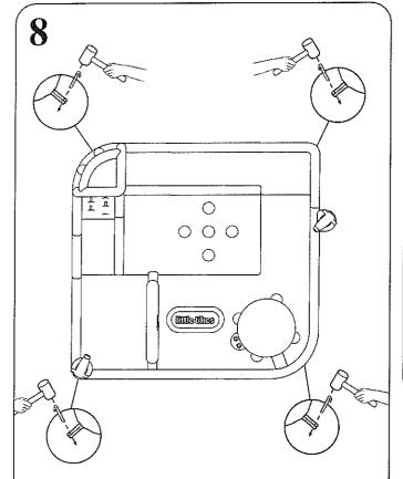
Secure the Water Park to the ground with the provided stakes To avoid tripping, pull the stake loops all the way out, then drive stakes completely into the ground.
