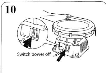
Once the Water Park is completely dry, turn off blower motor and unplug it from the outlet.
