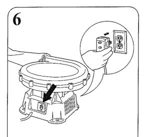
Switch power on. If blower does not operate when switched on, press reset button on GFCI adaptor
