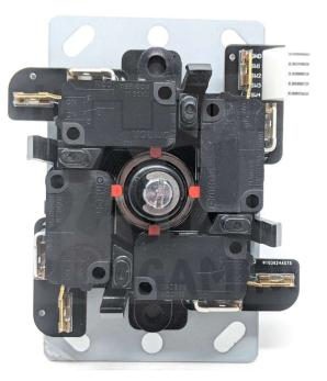
4. Place the joystick gate back onto the joystick housing. Once snapped in, the Shuriken JLF PCB will be firmly secured.
