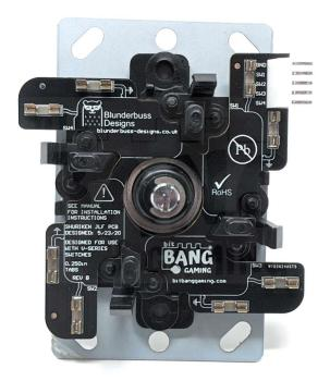
3. Carefully align each microswitch with the retention tabs. Make sure the microswitch terminals are between the retention tabs. The microswitches should naturally find its place when it aligns to the plastic pegs on the housing of the joystick. A firm push down will fully seat the microswitch.
