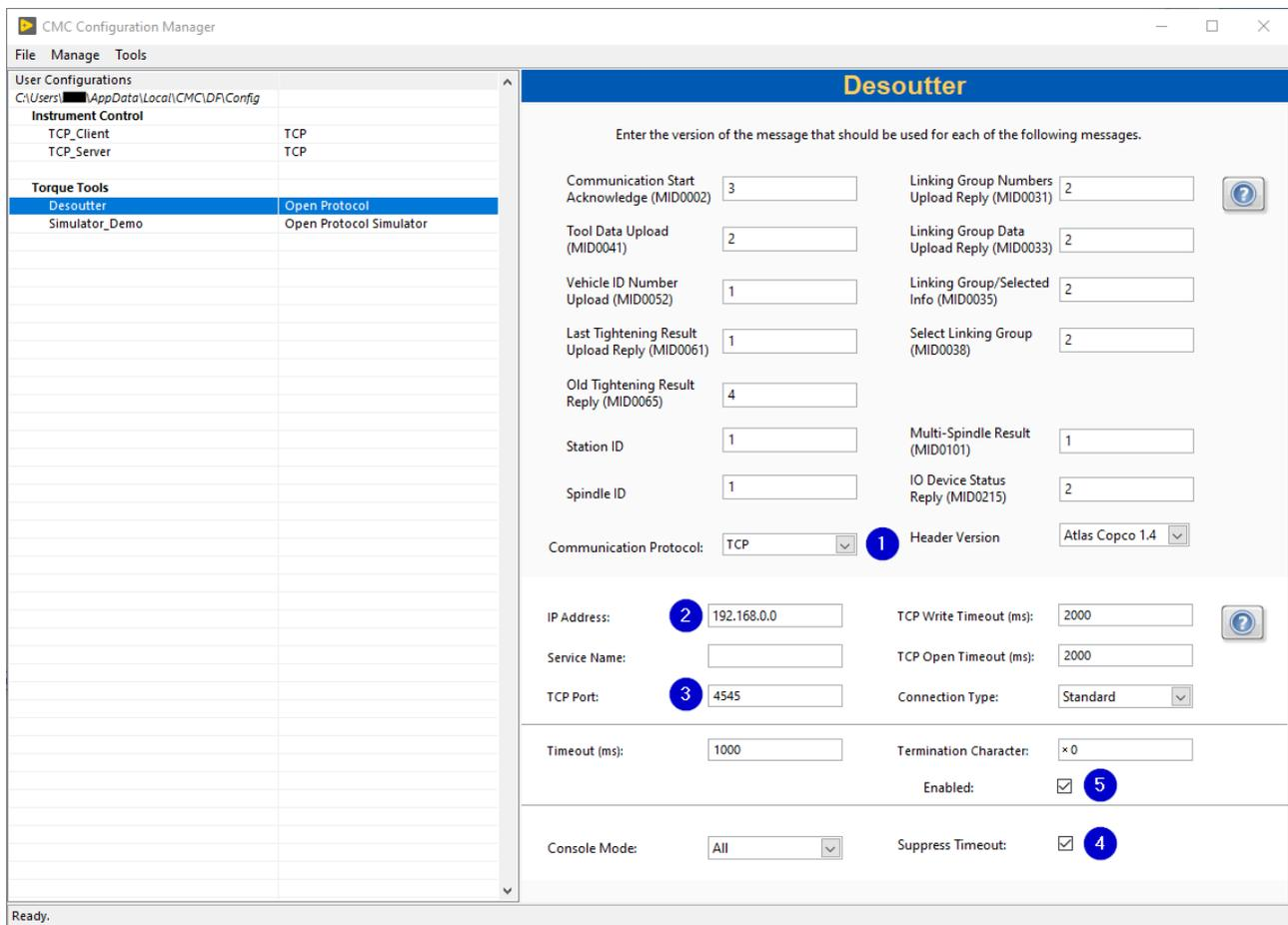
Figure 17. Open Protocol Torque Tool Configuration.
