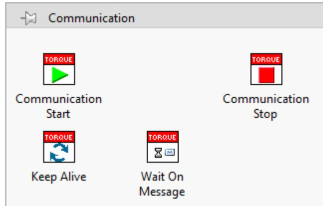
Figure 6: Torque Tools Communication Palette
