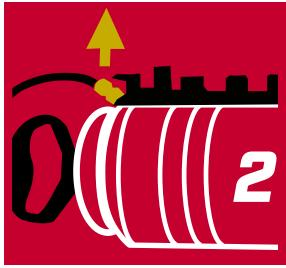
2 Tip sprayer upside-down, or on its side (with outlet tube at 12:00). Spray until only air is fully expelled
