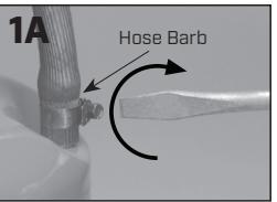
Make sure hose is pushed all the way to the tank. Make sure hose clamp is tight and below the hose barb. Turn clockwise with a screwdriver to tighten.
