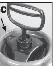
**TO LOCK HANDLE:** Push handle down to depress coil spring and turn handle 1/4 turn clockwise, then allow handle to raise into lock position.
