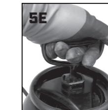
**TO RELEASE HANDLE:** Push down to depress coil spring and turn handle counterclockwise 1/4 turn, then lift handle.
