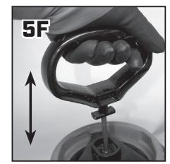
**TO UNLOCK PUMP:** Turn handle counterclockwise until 3-prong clamp is loose. Then rotate clamp counter-clockwise to stop 1/4 turn, then lift handle.
