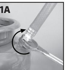
Attach the hose by screwing the swivel nut clockwise and tightening to 37 in. lbs. Refer to Pre-use check before using.
