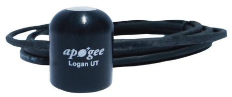
This silicon-cell pyranometer is calibrated to measure total shortwave radiation. The evaporation of water from soil and the transpiration of water from plant leaves are largely determined by the intensity of shortwave radiation, which is measured in Joules per meter squared per second or Watts per meter squared.
