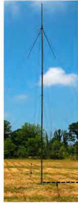
Four radio communication ports from one elevated antenna: 4 x VHF/UHF (30-88 or 225-450 MHz) * Simultaneous transmit or receive
