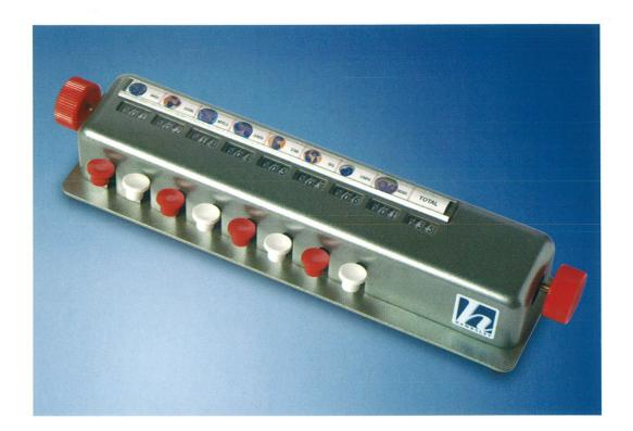
An intuitive differential cell counter that simplifies blood cell counts. When a total of 100 cells is counted, a bell rings. The percentage of each type of cell can then be read directly from the window above each key. A simple counter-clockwise rotation of the end knobs will zero all the counts.
