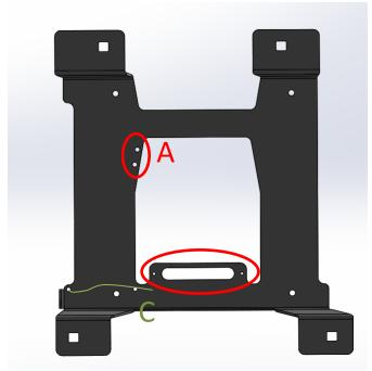
A – Fit Airbag Deployment Sensor here (see item 3 in image on previous page) using hardware from OEM seat B – Fit control box here (see item 11 in image on previous page) using hardware from OEM Seat C – Route wire from seatbelt buckle as shown, using OEM Clips
