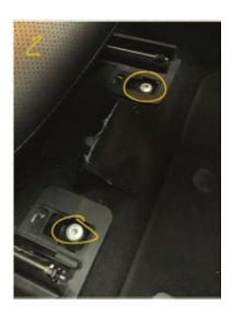
Undo and remove Front T50 Bolts
