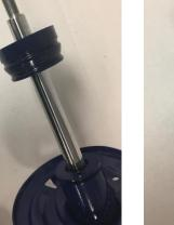
Use the provided o-rings on the REAR shocks below the bumpstops for lowered applications Steeda S550 Mustang Bumpstop Kit 555-4445
