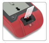
Place microcuvette into analyzer.
