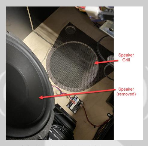
The speaker spacer in this kit will provide an additional ½ inch of clearance to keep the surround from hitting the speaker grill, thus eliminating vibration in the cabinet speaker.
