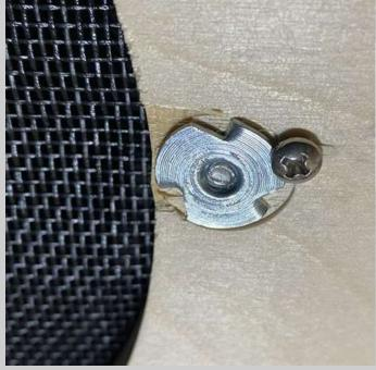
Remove the four Phillips head bolts holding the speaker down. You will need a short Phillips screwdriver to get the back bolt out or have an assistant help move the playfield so you can get to the bolt with a normal length screwdriver. Move the speaker out of the way while being carful not to damage the cone of the speaker.
