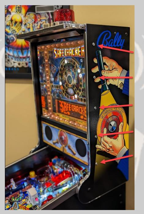
Install the left door panel as shown using the included black 8/32 x 3/4 machine screws (Item #3). If for some reason your machine does not have the factory holes on the back box you can use the included black sheet metal screws to attach the doors.
