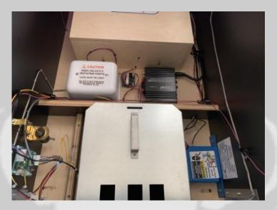
Using the included labels in the kit, carefully label the speaker wires and the terminals that they go to on the Lepai amplifier.
