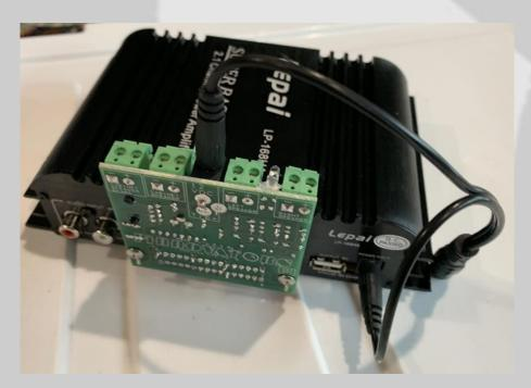
Insert the original speaker wires into the BBB. The BBB speakers and polarity are labeled on the back of the board. Insert the second subwoofer speaker wires into the second sub terminal block.
