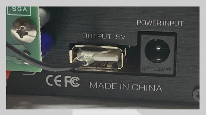
Insert the 12V power splitter cable into the power connector on the BBB and the power connector on the amplifier. Reinstall the amplifier into the cabinet. (Ground wire not shown)
