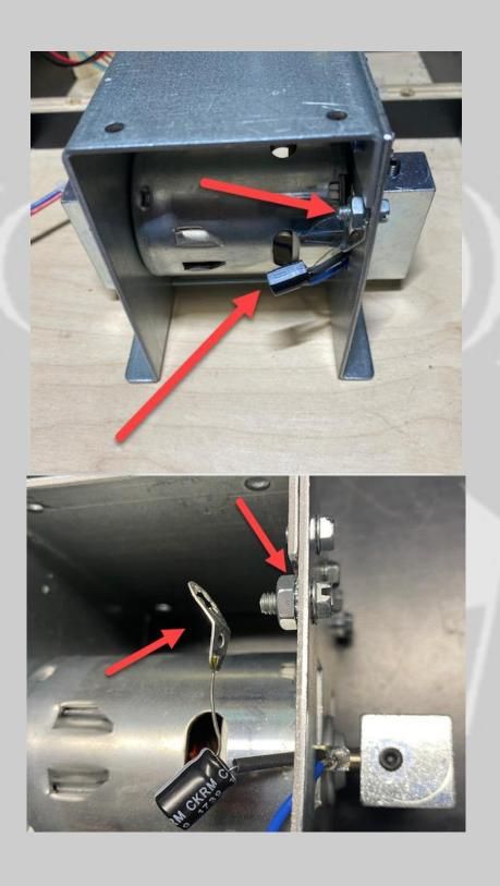
Next, trim off the other lead of the capacitor and then remove the capacitor completely.
