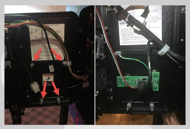
Insert the PinPAC9 plate as shown below. Position the ESD ground wire (the green wire) on the threaded stud. Fasten with the original hardware.
