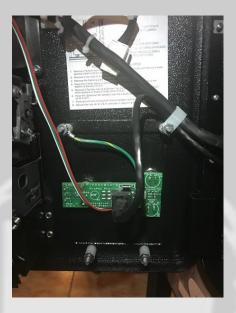
Insert the end of the RJ45 Cable into the connector on the PinPAC9 front control panel as shown.
