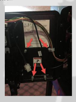
Insert the PinPAC9 plate as shown below. Position the ESD ground wire (green wire) on the threaded stud. Fasten with the original hardware.
