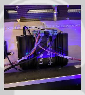
Insert the original speaker wires into the BBB. The BBB speakers and polarity are labeled on the back of the board. NOTE: This picture does not show all the labels on the wires.
