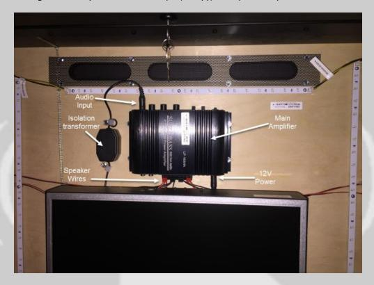
Take note of where the controls are set to on the amplifier. Use a cell phone camera to capture a picture.
