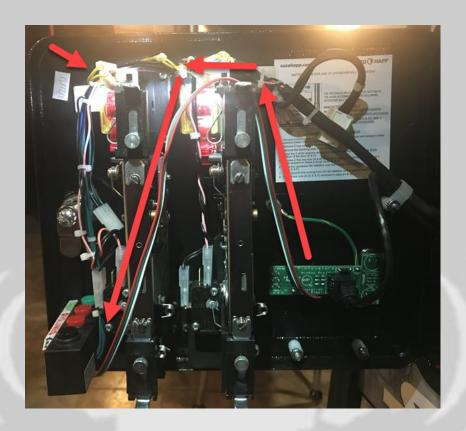
The MAC cable has a small printed circuit board (PCB) with connectors mounted to it. The PCB is inserted in line with the cable going to the coin door pushbuttons as shown below.
