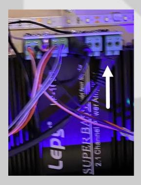
Plug the original amplifier power cable into the new power splitter cable.
