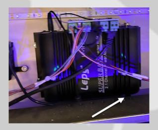
Plug the included 12 foot 3.5mm to 3.5mm cable into the gold jack on the BBB (Cable not shown)
