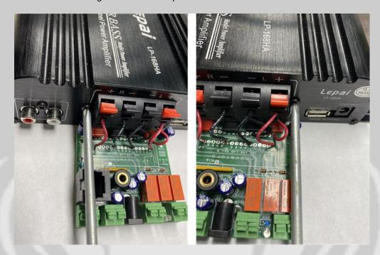
Using the included hardware, place one of the two spacers between the amplifier and the BBB. Insert one of the new screws through the BBB and then through the spacer. Tighten the screw a few turns to hold it in place.
