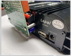
Insert the GROUND wires from the BBB into the space above the plastic part of the USB connector and the top metal frame of the USB connector. This wire gives the BBB an additional ground.
