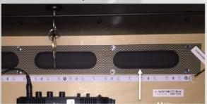
If you would like the cable to come out the bottom of the cabinet, look for an available vent hole on the bottom of the cabinet. Remove the fastener holding the screen and run the sub cable out the hole.
