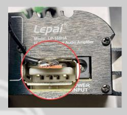
Insert the 12V power splitter cable into the power connector on the BBB and the power connector on the Amplifier.
