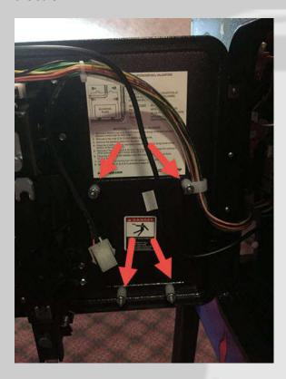
Insert the PinPAC9 plate as shown below. Position the ESD ground wire (the green wire) on the threaded stud. Fasten with the original hardware.
