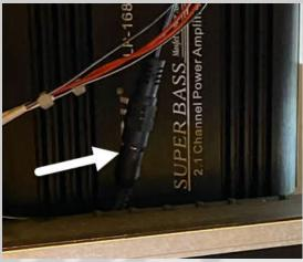
Reconnect the input audio cable to the Lepai. This is a 3.5 mm cable that was disconnected earlier.
