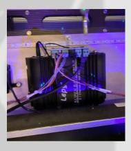
Insert the original speaker wires into the BBB. The BBB speakers and polarity are labeled on the back of the board.
