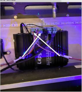
If the speaker wires do not reach the new speaker terminals once the amplifier is rotated, remove the cable ties on the speaker wires in the location shown below to allow more cable slack.
