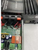
Using the included hardware, place one of the two spacers between the amplifier and the BBB. Insert one of the new screws through the BBB and then through the spacer. Tighten the screw a few turns to hold it in place.
