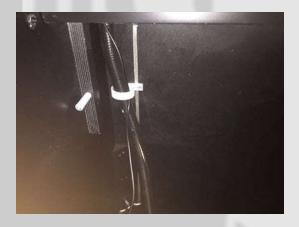
Continue to route the cable along the wire harness. Secure the cable in the white cable clamps. The cable will end up at the coin door.
