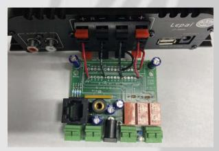
Unscrew the two screws to the right and left of the speaker terminal block.
