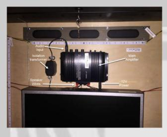
Take note of where the controls are set to on the amplifier. Use a cell phone camera to capture a picture.
