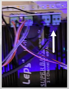
Plug the original amp power cable into the new power splitter cable.
