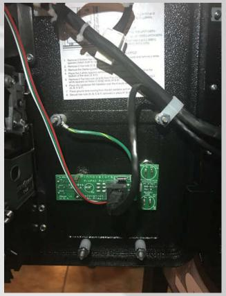
Insert the end of the RJ45 Cable into the connector on the PinPAC9 front control panel as shown.
