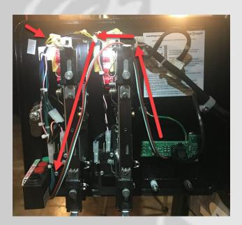
The MAC cable has a small Printed Circuit board with connectors mounted to it. The PCB is inserted in line with the cable going to the coin door pushbuttons as shown below.
