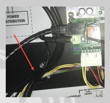
Run the cables down through the bottom of the back box and into the main cabinet.
