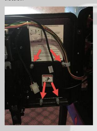
Insert the PinPAC4 plate as shown below. Position the ESD ground wire (the green wire) on the threaded stud. Fasten with the original hardware.
