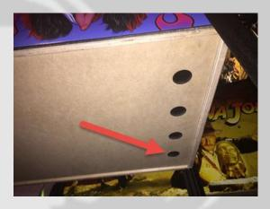
Finally, route the 3.5mm sub cable out the vent hole. Use the included Velcro tie to secure the cable to the leg of the pinball machine.
