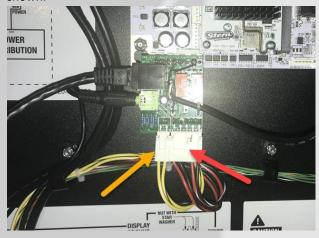
Plug (Optional accessory) Pinnovators 3.5 mm 12ft cable from the subwoofer cable kit into the 3.5mm green jack on the Back Box Board (BBB).
