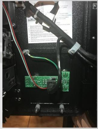
Insert the end of the RJ45 Cable into the connector on the PinPAC4 front control panel as shown.
