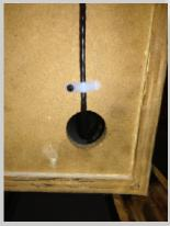
G. Using a helper, remove the playfield glass and lift up the playfield. Thread the control cable up through the cabinet and into the Back Box.
