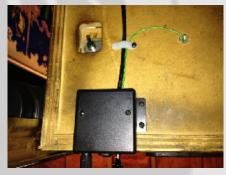
Wrap the exposed end of the wire on the exposed ground stud of the power box. Secure the wire to ground as shown using the supplied nut.
