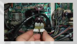
Insert the original Speaker cables on to the pins of the Back Box Board. Note: the connectors can go on either set of pins without causing damage and will function properly for this Back Board.
