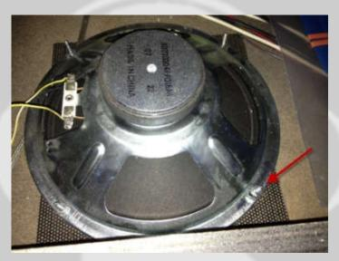
Form a hook on the end of the ground as shown. Place the hooked wire around the screw head as shown. Push the screw head up and then tighten the nut on the speaker until the wire is secured.
