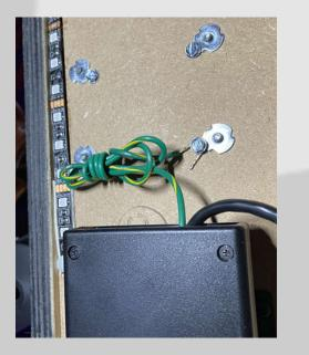
Ground Wire Method #4: Stern Spike games with NO shaker motor installed but has T-NUTS installed.
