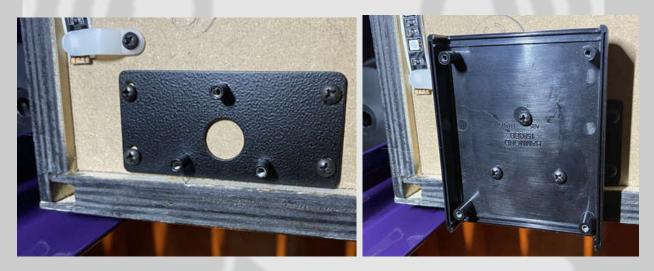
Carefully reinstall the bottom of the control box and fasten it with the 4 screws that were originally removed.
