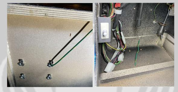
Fasten the ground wire to the ground braid as shown below.
