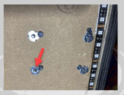
Loosen one of the screws that hold the T-NUT in place enough to wrap the ground wire around it. Wrap the ground wire around the screw and tighten the screw.
