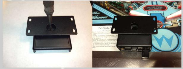
Position PinPac 3 under the cabinet and mount just the top half as instructed in the earlier section of this manual.
