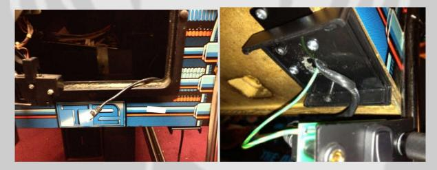
Plug the other end of the Control cable into the RJ45 connector in the box. Route the cable inside the box as shown. Assemble the box and route the cable inside the cabinet and up to the Back Box.
