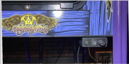
The PinPAC 10 control box is wider than the PinPAC 3 box. The mounting screws are not 100% accessible so the control box must be disassembled before mounting.
