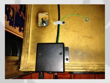
Wrap the exposed end of the wire on the exposed ground stud of the power box. Secure the wire to ground as shown using the supplied nut.
