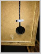
F. Using a helper, remove the playfield glass and lift up the playfield. Thread the control cable up through the cabinet and into the Back Box.
