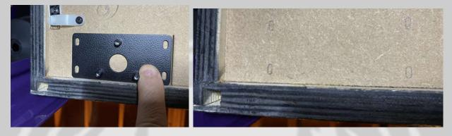
Mount the bracket as shown using 4 of the black screws. Remount the top cover.
