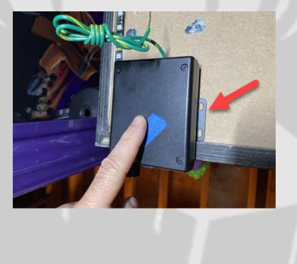
Remove the 4 screws that hold the top and bottom covers together on the control box. Separate the top cover from the rest of the unit.
