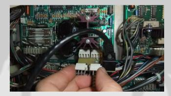
Insert the original speaker cables on to the pins of the Back Box Board. Note: the connectors can go on either set of pins without causing damage and will function properly for this Back Box Board.
