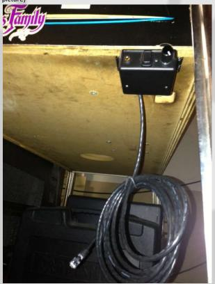
B. Place the PinPac3 box bracket up against the front face of the machine. Using a pencil, mark the slots where the mounting screws will go. Make sure your happy with the placement. (Have someone hold the PP3 box for you while you take a final look)
