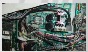
Feed the remaining cable down the bottom of the Back Box and into the cabinet.
