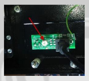
This trim pot has different functionality depending on the Back Box Board type. The main purpose was to allow the user to "Mix" the Cabinet speaker channel and the Back Box Speaker channels going into the headphones. The trim pot provides a reasonable amount of mix on most of the boards. Note that the WPC-Dot Matrix system really only has ONE channel so the trim pot can't adjust the mix, just the overall level in the headphones.
