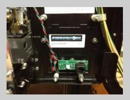
Route the PP2MAC remote cable over the top of the coin slots as shown. Route it down to the system control panel buttons. *NOTE: The three color cable is now a flat three color ribbon cable.*
