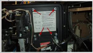
Insert the PinPAC1 plate as shown below. Position the ESD ground wire (the green wire) under the nearest available threaded stud. Fasten with the original hardware.
