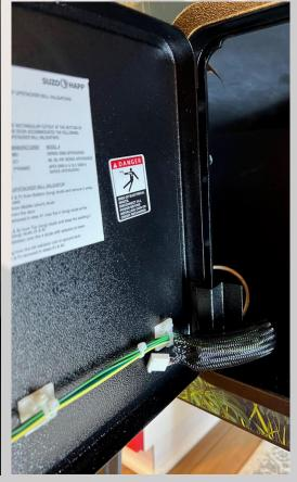
Secure the cable to the door wire harness. There are two possible ways. You can snip the cable tie on the mounting pads and then resecure the cable harness with the new Pinnovators cable using the included cable ties.
