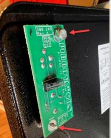
Insert the Pinnovators cable into the keyed connector on the back of the control panel. Fasten the wire ties completely now.
