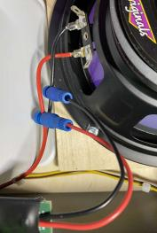
Guns n Roses (CE) provides a nice subwoofer cable exit in the vent hole.
