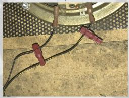
Insert the wires from the PINsub MS into the hole in the small endcaps. Carefully twist the small endcaps until finger tight.
