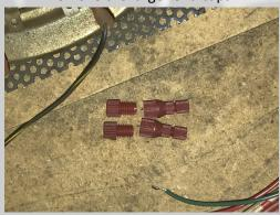
Place the large endcaps over one of the two speaker wires.
