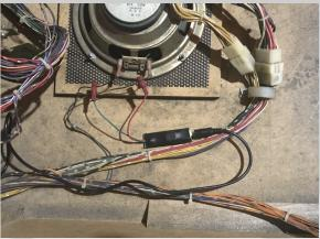
Locate the vent hole in the right rear of the cabinet. Push up on the vent screen to dislocate it to allow the 3.5 mm cable to be fed down through the vent hole.
