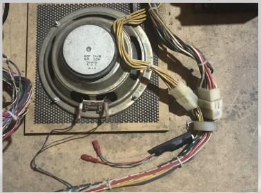
Remove the two PosiTaps by twisting the smaller end cap.
