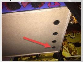
Secure the cable into the nylon cable clamp to protect the cable from being pulled out. The nylon cable clamp does not have to be removed to get the wire into it. The clamp can be slightly stretched open.
