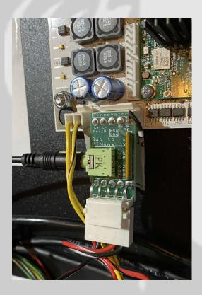
Insert the original Speaker cable on to the pins of the Back Box Board.
