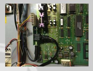
Using the 12 foot 3.5mm to 3.5mm supplied cable, poke the cable through the air vent located above the main CPU board as shown below.
