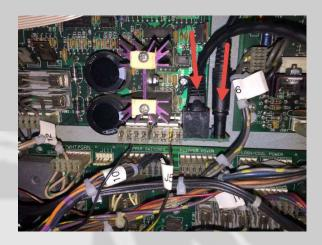
Using the 12 foot 3.5mm to 3.5mm supplied cable, poke the cable through the air vent located above the main CPU board as shown below. Loosen the screws on the vent to allow the cable to exit.
