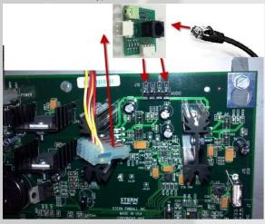
Insert the Back Box Board into the speaker connectors on the sound card as shown above. Make sure it's fully inserted and aligned properly.
