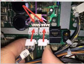
Note: The PINsub\_DM kit will not have the black RJ45 connector loaded so you will not have an RJ45 cable. The cable is part of the Pinnovators headphone kit.
