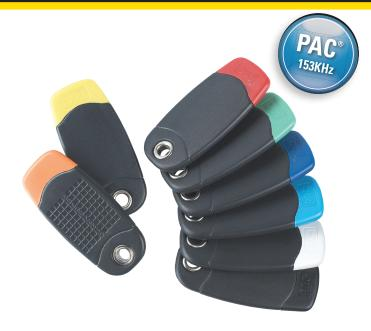
The passive proximity technology in the PAC token requires no batteries or physical contact with the reader; this helps assure that the tokens are virtually wear-free and will provide years of service with no maintenance backed by a lifetime guarantee against electronic failure. Robust, world-class construction combined with advanced technology, incorporating a pre-programmed unique identification number without site codes, makes programming easy and copying almost impossible.
