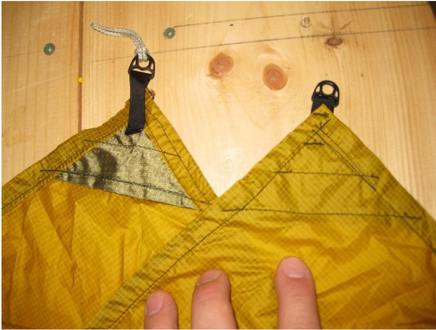
Back (left) and Face (right) of ground tie-out
