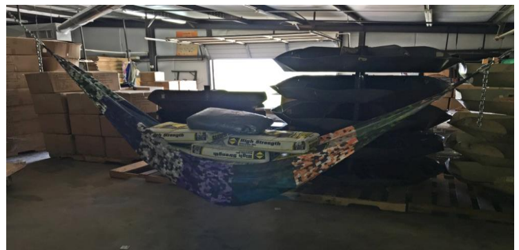
Static Load Test Setup (reference)
