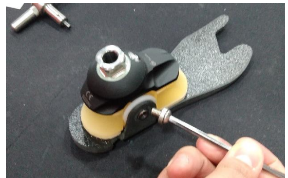
Figure 14: Installing the screw and washer
