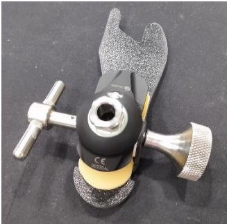
Figure 12: Bullet inserted into shaft guide
