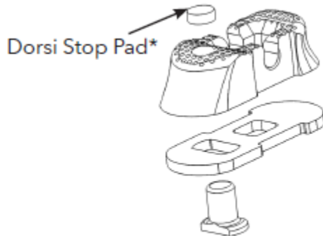
Figure 5A: Kinetic Edge Dorsi stop inserted into pad spacer, bumper and dorsi stop pad
