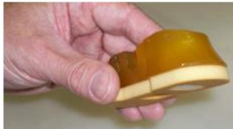
Figure 5B: Dori stop inserted into pad spacer and bumper
