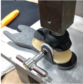
Figure 11: Pushing the axis assembly through the ankle joint
