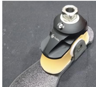
Figure 9: Upper bracket inserted into foot cavity
