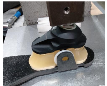
Figure 10: Upper bracket being compressed
