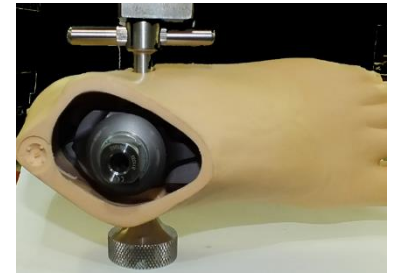
Figure 103B: Fully seating the axis
