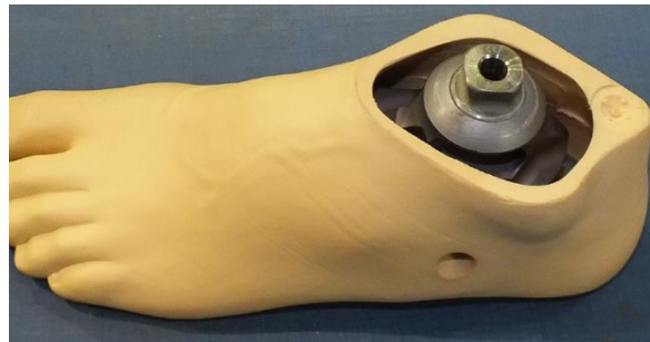
Figure 9B: Upper bracket inserted into foot cavity
