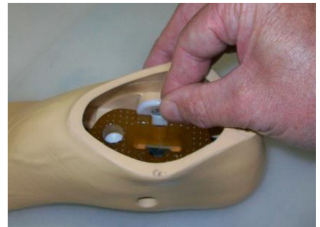
Figure 5: Insert Bumper Assembly
