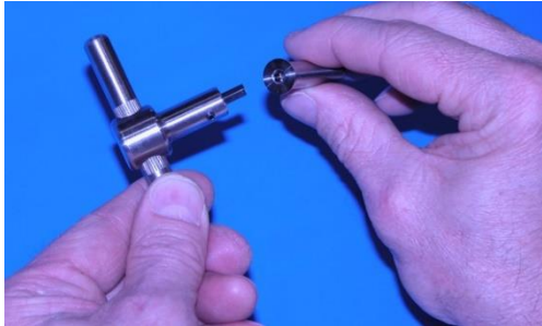
Figure 7A: Insert hex shaft driver into shaft
