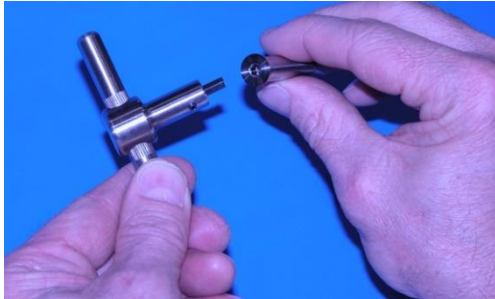
Figure 7A: Insert hex shaft driver into shaft
