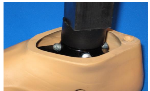
Figure 10: Upper bracket being compressed
