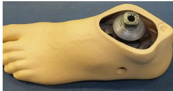
Figure 9B: Upper bracket inserted into foot cavity
