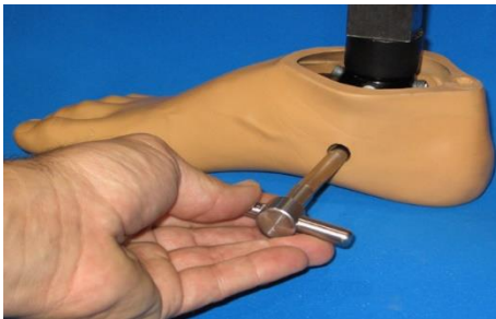
Figure 18A: Pushing the axis assembly through the ankle joint
